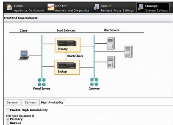
The IBM Security Web Gateway Appliance displays how high availability and workload distribution for the virtual appliance is provided by an integrated front-end load balancer.
